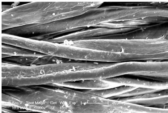
**Figure 2: Scanning Electron Photomicrograph of Benzophenone-2 Treated Cotton Fabric at 20  $\mu\text{m}$**
