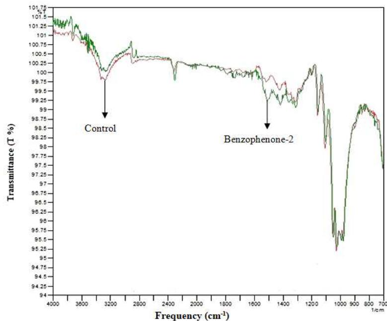
**Figure 3: FTIR of Untreated and Benzophenone-2 Treated Cotton Fabric**
