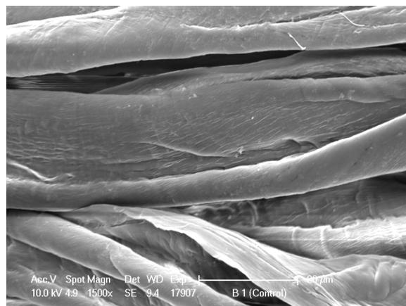
**Figure 1: Scanning Electron Photomicrograph of Untreated Cotton Fabric at 20 μm**
